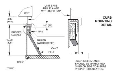
Roof Curb kits ship dis-assembled for ease of handling and storage. All kits ship complete with mounting hardware (for unit to curb), insulation, gasketing, sealant and installation instructions for field mounting.
